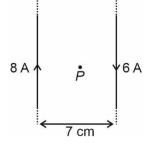
P is equidistant from the wires find magnetic field at point P. (Point P is in the plane of wire)
