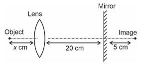
The image shown is formed after refraction from lens and reflection from mirror. If the length of lens is 10 cm, find x.
